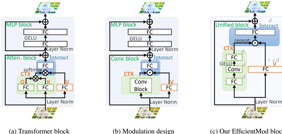
Figure 1: Comparison of Transformer, abstracted modulation design, and our EfficientMod block.  $\otimes$  is element-wise multiplication and  $\otimes$  means matrix multiplication. Compared to Transformer and abstracted modulation, our unified block efficiently modulates the projected values ( $V$ ) via a simple context modeling design (CTX). Dimension number is indicated in (c) to aid comprehension.
