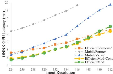
Figure 8: Impact of input size on GPU latency.
