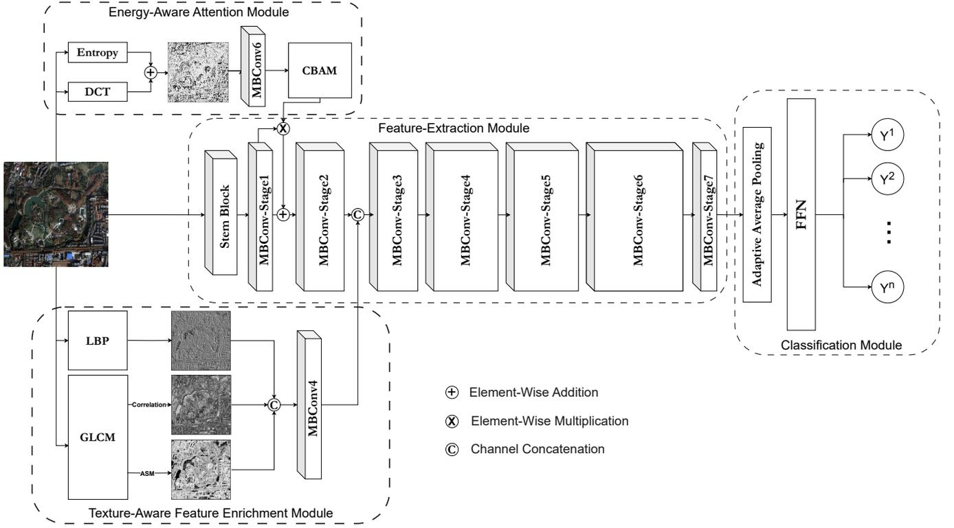
Fig. 1. Overall Architecture of the proposed Network comprised of the following modules-TAFEM,EAAM,FEM and CM.
