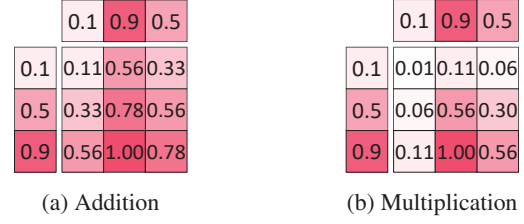
Fig. 3: Multiplication fusion produces a sharper peak value and smaller focus region than addition fusion. The output values are normalized after fusion.
