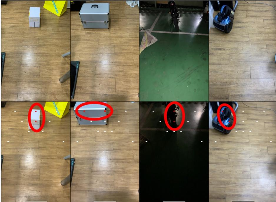
Fig. 8: The upper images illustrate situations with obstacles in the front. The bottom images visualize the execution of the pedestrian assistance system in the upper environment. It can be observed that when the assistance system is activated, obstacles in the front are detected, and the points change to red.
