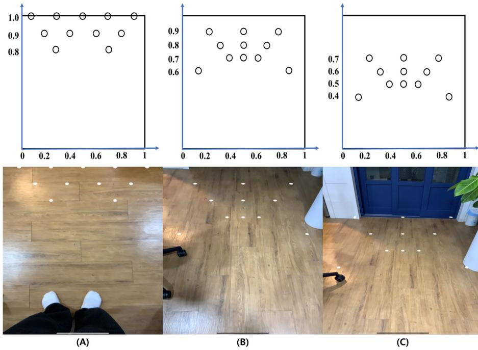
Fig. 7: The upper graph represents the normalized coordinates (ranging from 0 to 1) of a smartphone screen in both horizontal and vertical dimensions. The white points on the graph denote the detection positions of LiDAR. The lower image illustrates the application of these white points from the graph onto the actual screen.
