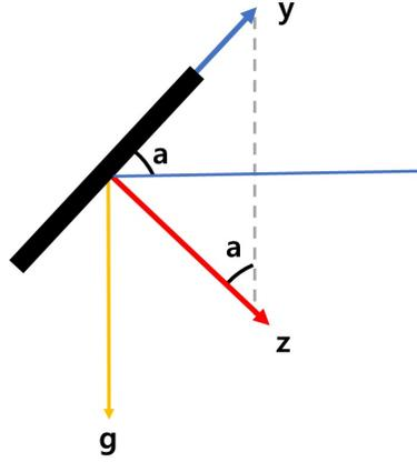
Fig. 5: This illustration depicts the accelerometer axes and angles on a smartphone. The black rectangle represents the smartphone. The angle can be obtained using the z,y values of the accelerometer
