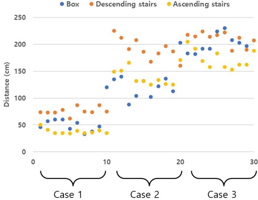
Fig. 9: This graph displays the distances measured between obstacles and pedestrians in various scenarios. The cases are categorized based on the device angles, revealing that as the angle increases, the measured distances also become longer.
