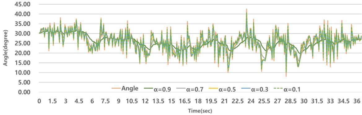
Fig. 10: This graph illustrates the variation in angles with different  $\alpha$  values when utilizing a low-pass filter.
