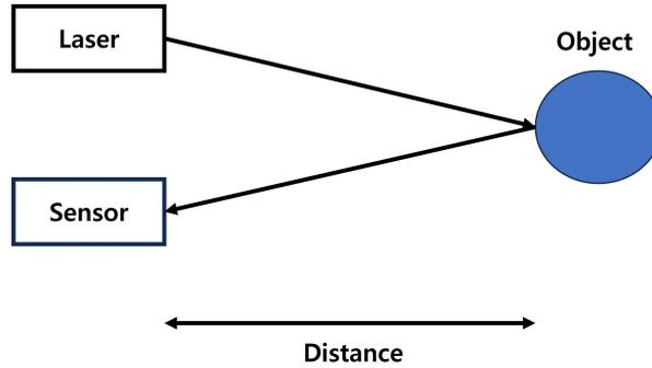
Fig. 3: The measurement technique of dToF (direct Time-of-Flight) uses the time it takes for the emitted light from a Laser to be detected by the Sensor, enabling the calculation of distance.
