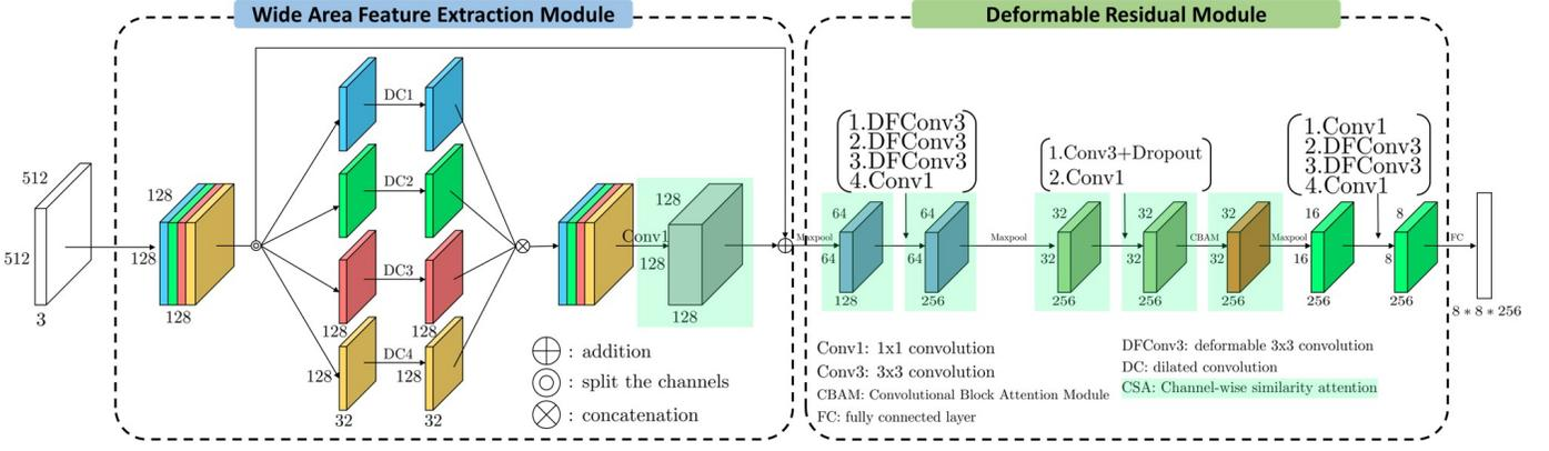
Fig. 1: Overall architecture for vehicle state classification. There are two parts, WAFE module, wide area feature extraction, and DR module, deformable residual module. CSA: Channel-wise similarity attention in the green box.
