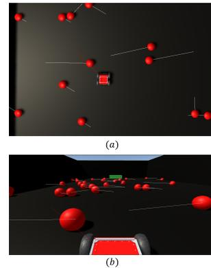
Fig. 5: The environment of experiments. The line segment from objects represents the velocity. (a) Top view of environment. (b) View from the robot.
