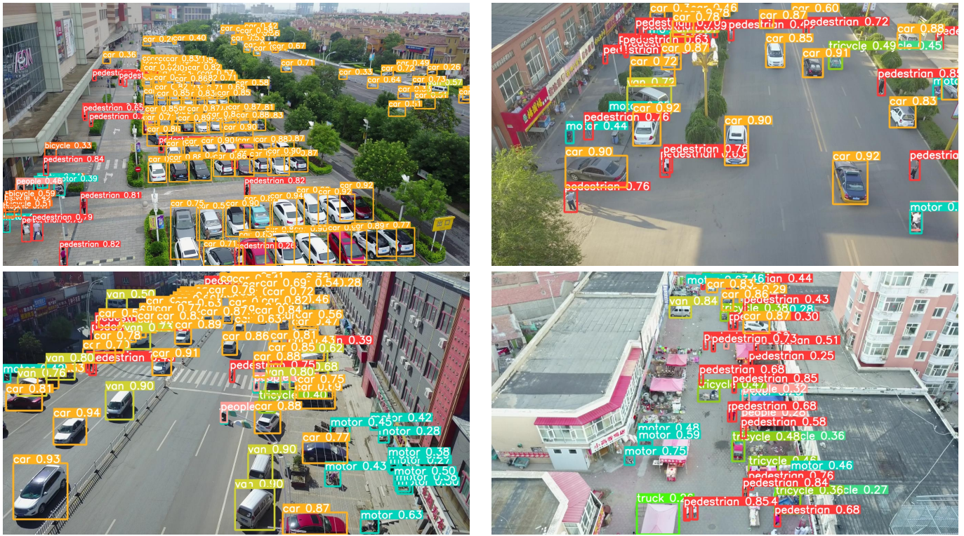
Fig. 6: Object Detection Result on VisDrone 2019 dataset.
