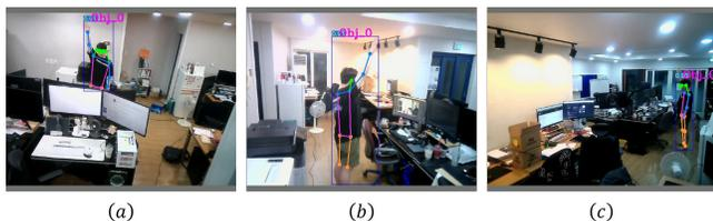
Fig. 7. Pose estimation from (a) camera 1, (b) camera 2, (c) camera 3.
