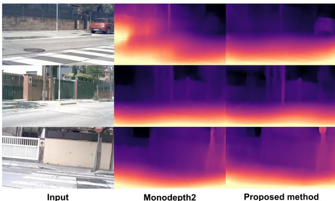
Fig. 6: This is the output depth images of Monodepth2 and the Proposed method. When comparing the Proposed method's images with Monodepth2, it is evident that the boundaries of objects are more distinct.
