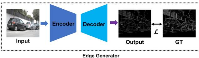
Fig. 3: Structure of Edge Generator. The Encoder compresses the input image using convolution and max-pooling layers and the Decoder restores the compressed image using two transposed convolution layers with ReLU activation. Output channel is set to 1.
