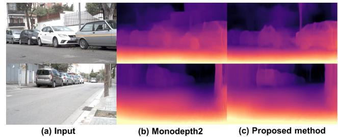
Fig. 1: The input images were sourced from the BIPEDv2 [2] dataset. In the original Monodepth2 image (b), there is a slight blurring of the boundaries of car, whereas in the proposed method image (c), the car's boundaries are more distinct and clear.
