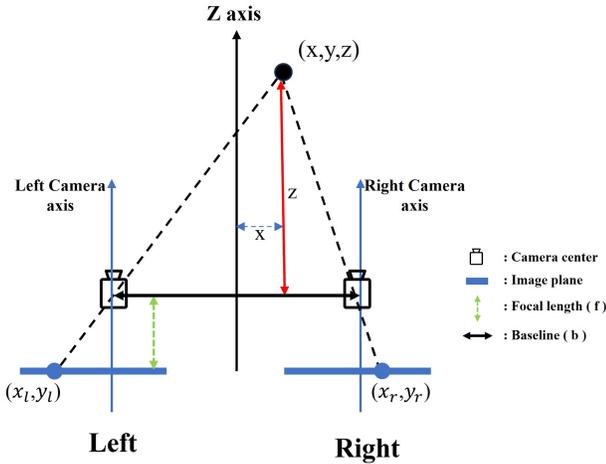
Fig. 2: This illustration depicts the depth estimation of stereo vision. The point  $(x, y, z)$  in 3D space is projected onto the left and right image planes through the camera lenses. The horizontal and vertical distances from each camera axis to the projected points are represented by  $(x_l, y_l)$  for the left image plane and  $(x_r, y_r)$  for the right image plane, respectively. Focal length is distance between image plane and camera lens. Baseline is stereo camera interval.
