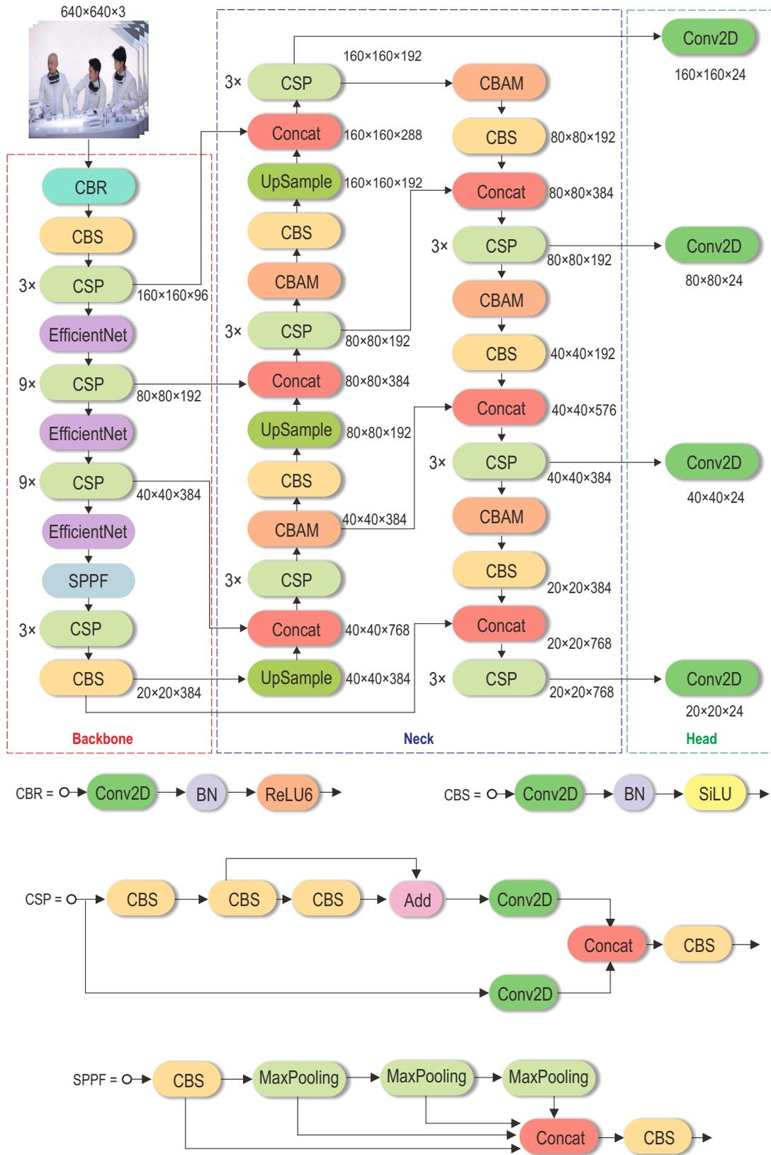
Fig. 1. The proposed network architecture overview and sub-modules.
