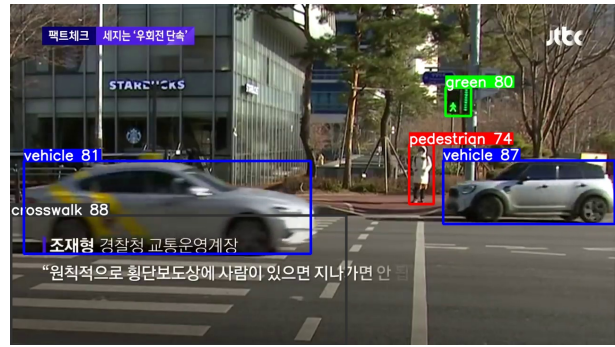
Fig. 5. Classified as general vehicle because there is pedestrian who is not crossing the crosswalk [12]
