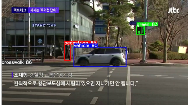
Fig. 7. Vehicle covers a pedestrian at the point of view of the camera
