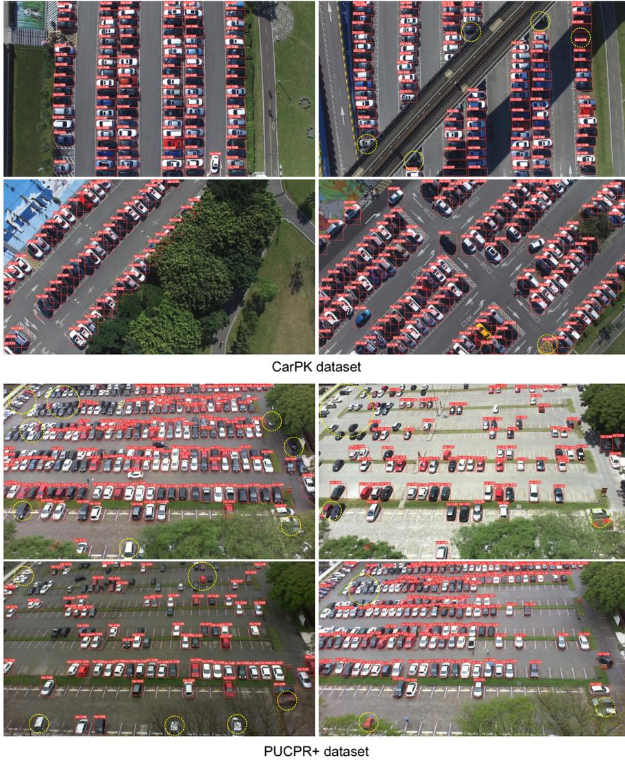
**Fig. 5.** The qualitative results and several mistakes of the proposed network on the validation set of the CarPK and PUCPR+ datasets with IoU threshold = 0.5 and confidence score = 0.5. Yellow circles denote the wrong detection areas.
