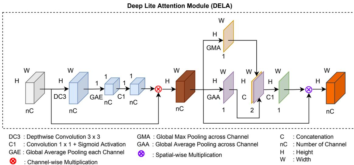
Fig. 3. The proposed Deep Lite Attention Module (DELA).
