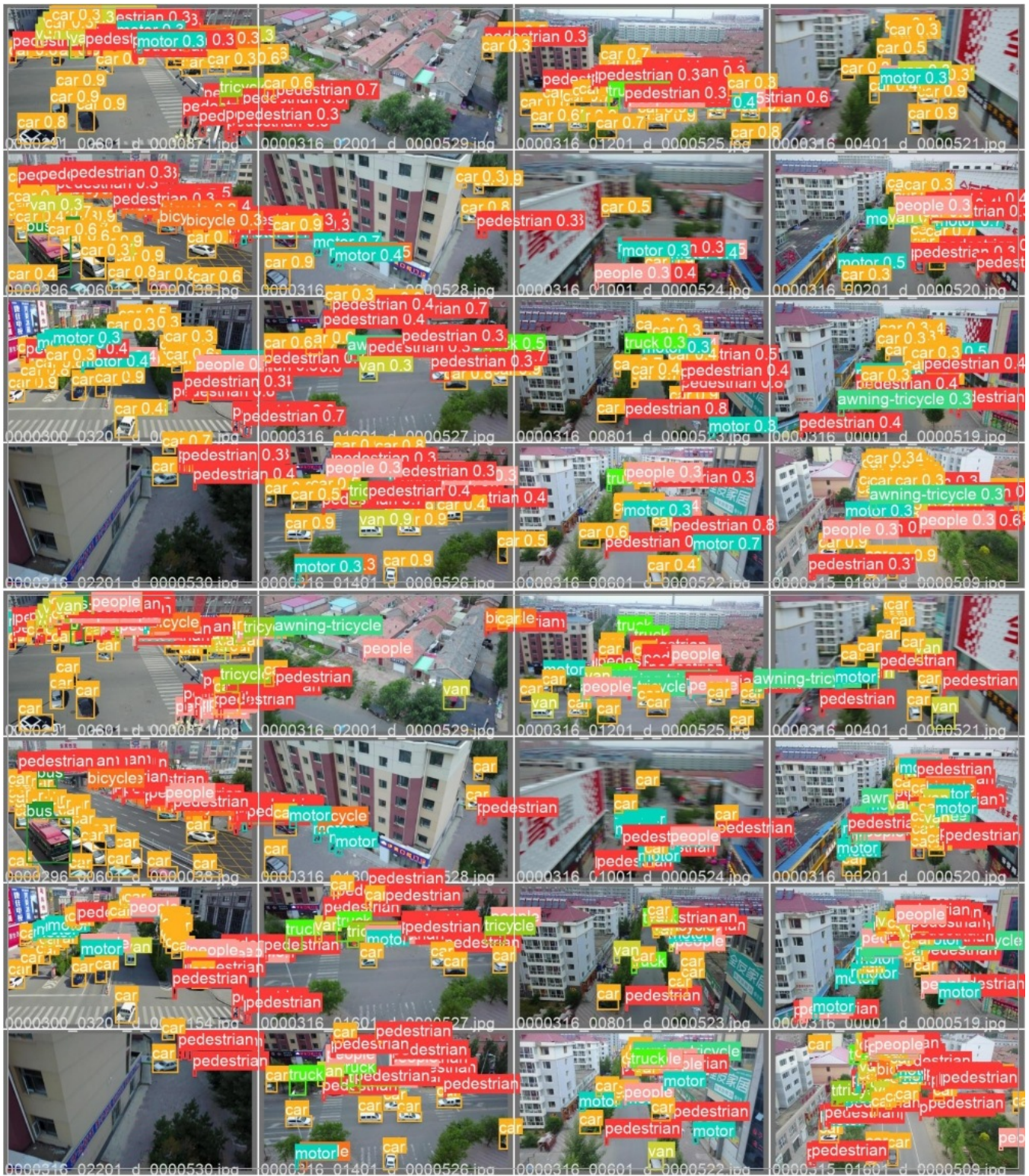
Fig. 5. Visualization of Prediction and Ground-truth Result on VisDrone Dataset
