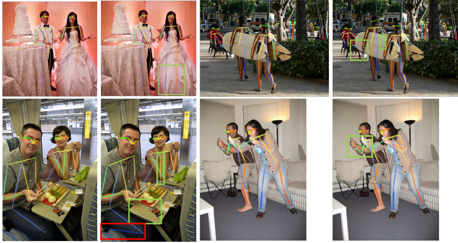
Fig. 5. Qualitative images for human pose estimation in COCO2017 test-dev set. In two similar images, the Right side is the result of the original human pose estimator HRNet-W32, and Left side is our approach. Greenbox means better keypoint detection than normal. Redbox means inaccurate keypoint detection.
