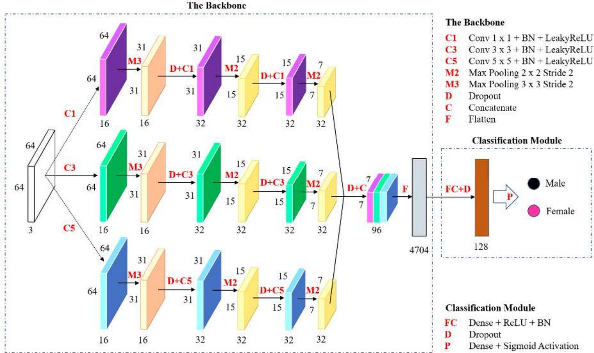
Fig. 1. The MPCConvNet architecture for gender recognition.
