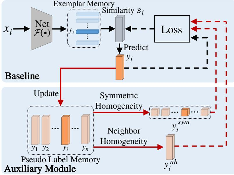
Fig. 1. The framework of our proposed SNNNet. The black line indicates the baseline network. Apart from the predicted main pseudo label  $y_i$ , we proposed an auxiliary module to seek auxiliary labels  $y_i^{sym}$  and  $y_i^{nh}$  as additional supervisions to optimize the network.
