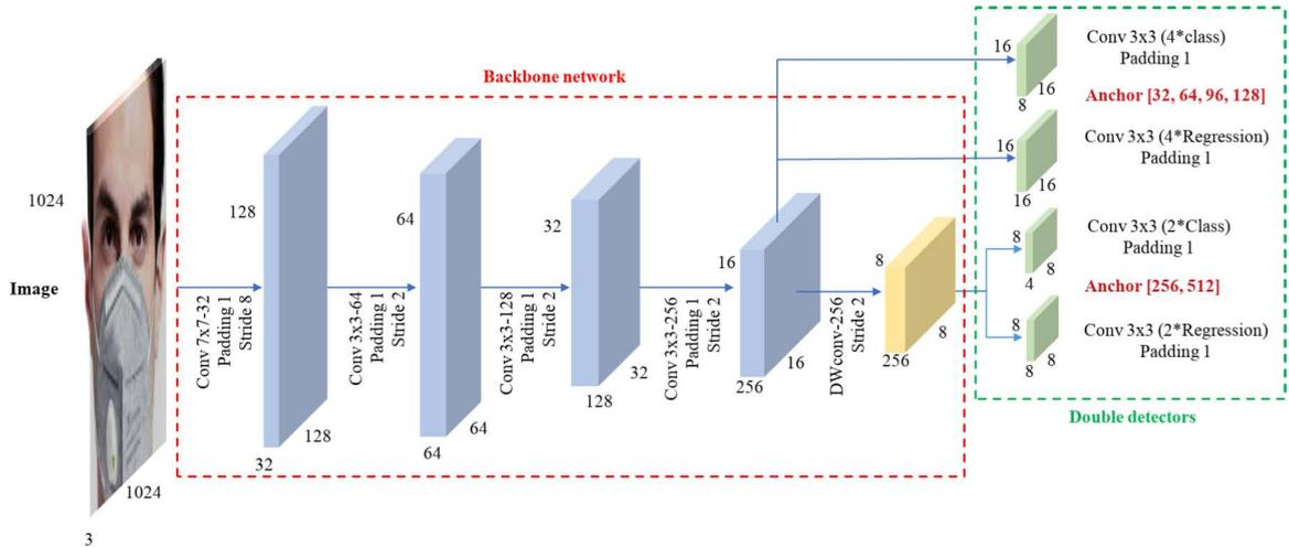
FIGURE 2. Structure of the proposed face detection network. It consists of a backbone network and double detectors.
