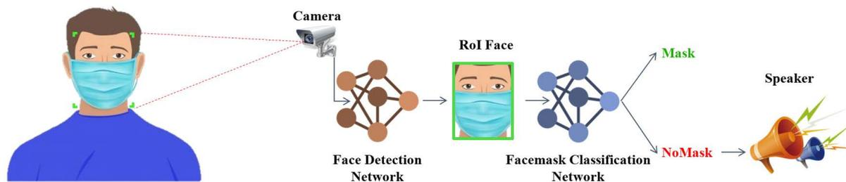
**FIGURE 1.** Overview of the proposed facemask wearing alert system. It consists of two stages: face detection and facemask classification.
