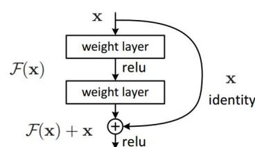
FIGURE 4. Structure of the skip connection layer [19].
