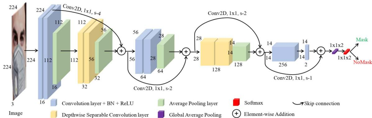
FIGURE 3. Structure of the proposed facemask classification network which consists of a stem, skip connection, and classification modules.
