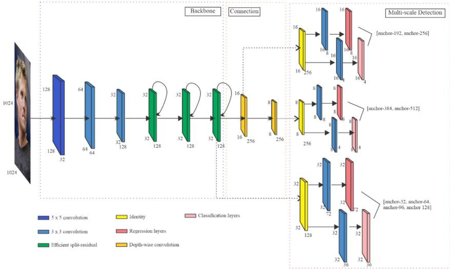
**Fig. 1.** The proposed architecture of face detector. It uses a combination of  $1 \times 1$  and  $3 \times 3$  convolution as extractor features. Multilayer detection with anchors assignment plays a role in predicting faces at various scales.
