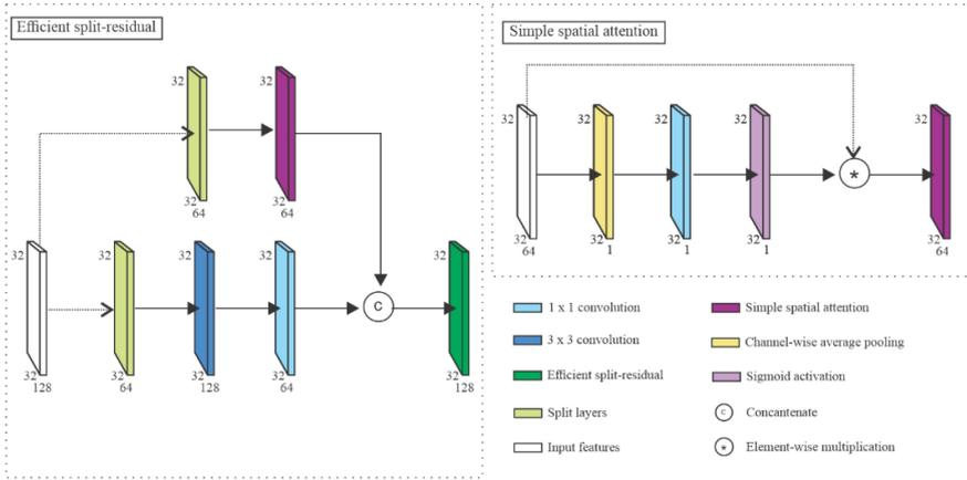
**Fig. 2.** The efficient split-residual as a stem module that sequentially extracts features and produces a few parameters and low-cost computation power (a). Simple spatial attention is employed at part of the input feature map to capture the representation of the valuable elements (b).
