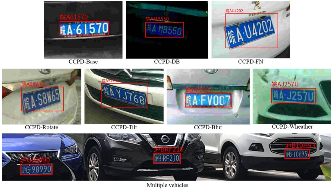
Fig. 4. The qualitative result of license plate detection and recognition system on CCPD dataset.
