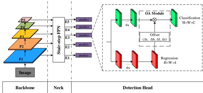
**Fig. 1.** The overall architecture of the proposed method includes the backbone, neck, and detection head. Stair-step FPN takes five feature maps ( $P_1, P_2, P_3, P_4, P_5$ ) as input and then obtains balanced features ( $E_1, E_2, E_3, E_4, E_5$ ). Offset Adaption OA Module takes four offset values and classification features as input.  $\otimes$  denotes  $3 \times 3$  deformable convolution.
