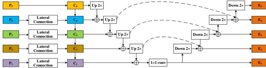
**Fig. 2.** The detailed architecture of the Stair-step FPN includes a top-down pathway and a down-top pathway. Up 2 $\times$  denotes Up-sampling operation with scale 2. Down 2 $\times$  denotes Down-sampling operation with scale 2.  $\oplus$  denotes summation operation.
