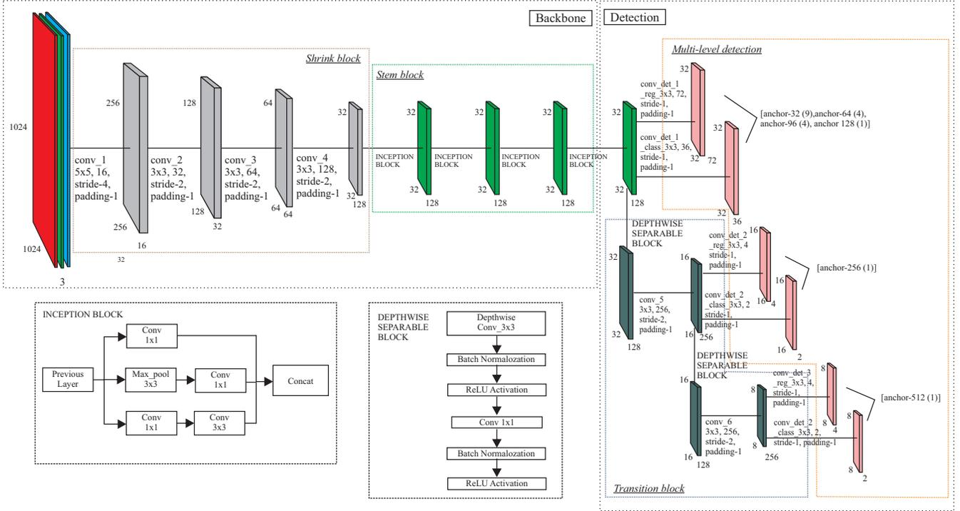
Figure 1. The proposed architecture consists of two main modules of the backbone to extract facial features using CNN and a multi-level detector to predict faces on multiple scales. Inception is applied to the stem block as a crucial module. The architecture consists of 30 layers of CNN and produces one million parameters.
