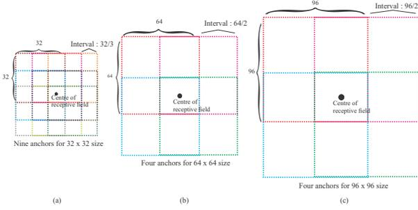
Figure 2. Examples of anchor densification strategies for anchor types are  $32 \times 32$  (a),  $64 \times 64$  (b), and  $96 \times 96$  (c). The anchor unit is in color. The anchor interval shows the distance between neighbor anchors of the same type.
