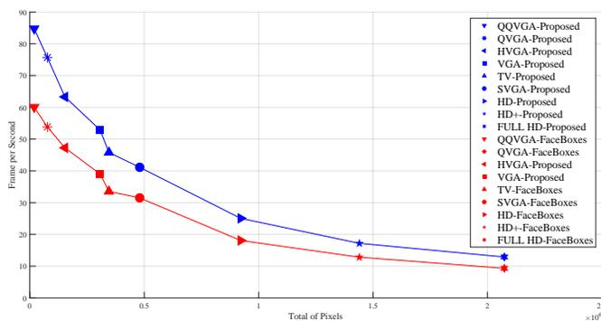
Figure 7. Comparison of detector data processing speed at different video input sizes.
