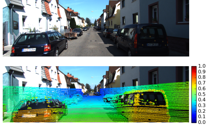
Figure 2: The top image is the original RGB image and the bottom one is the RGB D image. Red color means the depth is shallow, and blue color means the depth is deep. Best viewed with color.
