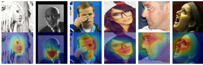
Fig. 2. Some challenging faces and their corresponding class activation maps (CAMs) [8] learned by LS-CNN model. Faces are influenced by illumination changes (Columns 1, 2), occlusions (Columns 3, 4), and pose variations (Columns 5, 6). MTCNN [13] fails to detect landmarks, while our LS-CNN model can locate discriminative face regions (Row 2).
