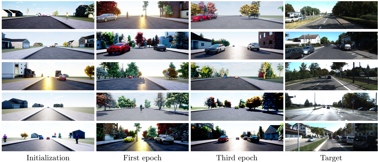
Figure 3. As the self-learning loop progresses, synthetic data increasingly matches the content of the target image. From left to right: synthetic data initialized by SDR [41], after first and third epochs, and corresponding real KITTI target images.
