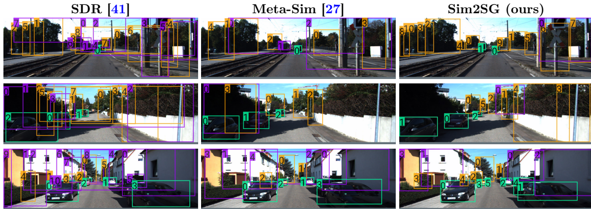
Figure 5. Qualitative results of objects detected on three different KITTI images. Left: SDR fails to detect many objects and yields a large number of false positives (mislabeled), leading to poor scene graphs (not shown). Middle: Meta-Sim improves on false-positives, but still fails to detect some objects. Right: Our method detects objects correctly with fewer false positives, thus generating more accurate scene graphs. (Cars in green, vegetation in yellow, buildings in purple.)
