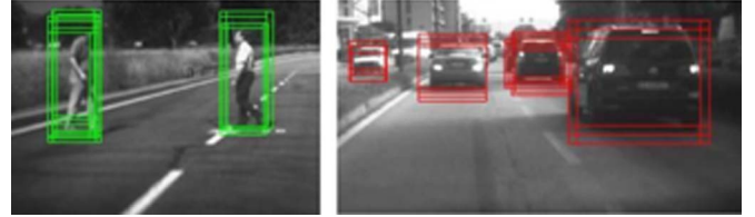
Fig. 7. Examples of successful detections of pedestrians (left) and cars (right) from camera images.
