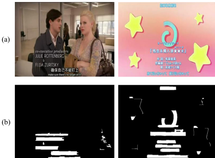
Fig. 3 Text region localization. (a) Original color images, (b) Candidate Text Regions Maps (CTRM)
