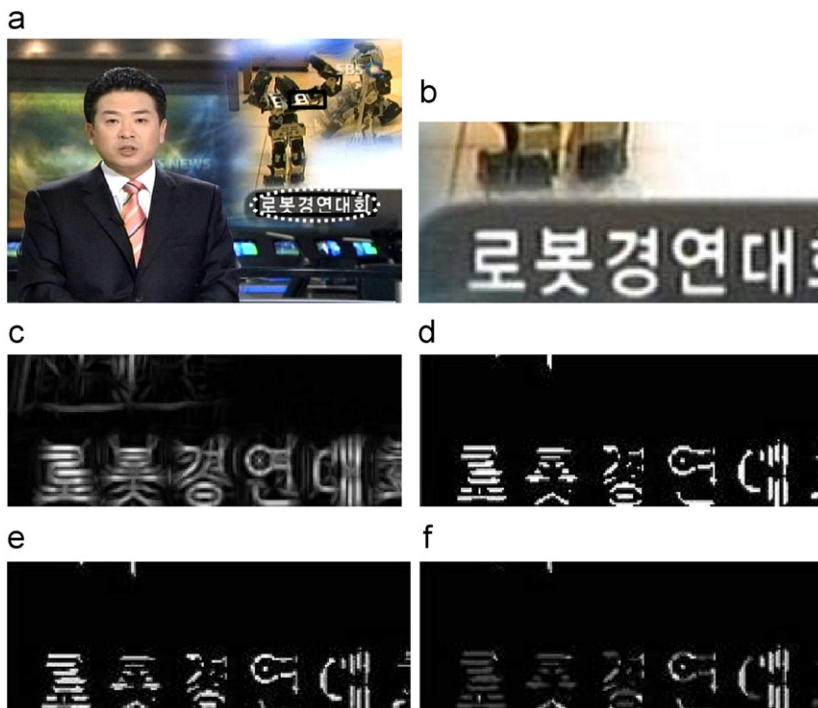
Fig. 4. Intermediate results by a stroke filter in a real text image: (a) original image, (b) text image, (c) stroke response map, (d) binarized map of (c), (e) stroke width map, and (f) stroke orientation angle map.
