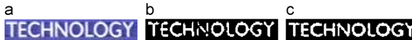
Fig. 7. Test examples: (a) source image, (b) binarized stroke response map, and (c) the local region growing result.
