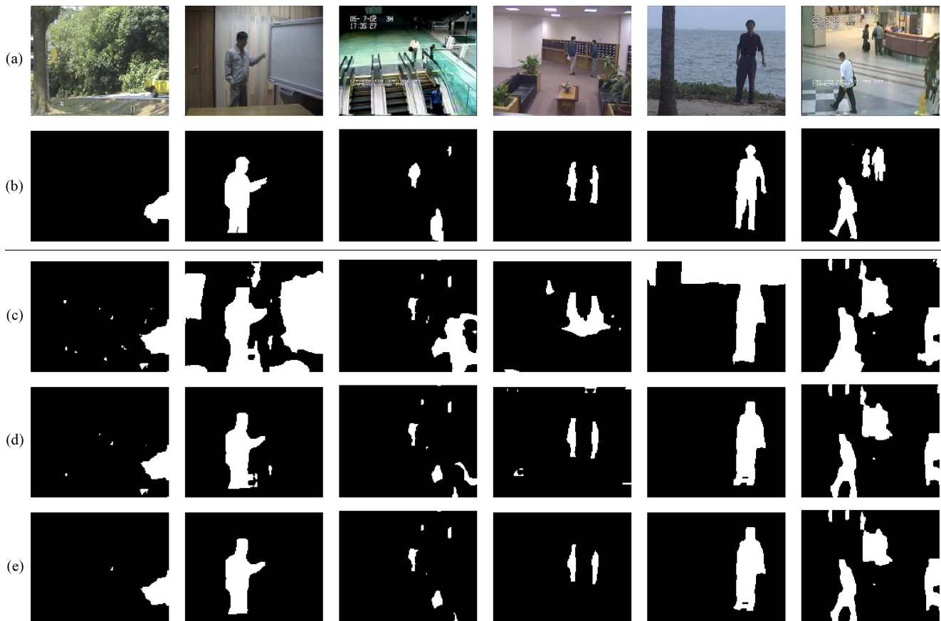
Fig. 4. (a) Example frames from I2R dataset. (b) Ground truth foreground masks. Foreground masks obtained by the proposed method using (c) the first classifier only, (d) combination of the first and second classifiers, (e) using all three classifiers. Adding the second classifier considerably improves the segmentation quality, while the addition of the third classifier aids in minor reduction of false positives. See Fig. 5 for quantitative results.
