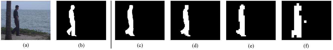
Fig. 2. (a) Example frame from the I2R dataset. (b) Its corresponding ground-truth foreground mask. Using the proposed method with a block size of 8 \times 8 , the foreground masks obtained for various degrees of block advancement: (c) one pixel, (d) two pixels, (e) four pixels, and (f) eight pixels (i.e., no overlap).
