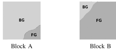
Fig. 1. Without taking into account block overlapping, misclassification is inevitable at the pixel level whenever a given block has both foreground (FG) and background (BG) pixels. Classifying Block A as a background results in a few false negatives (foreground pixels classified as background), while classifying Block B as a foreground results in a few false positives (background pixels classified as foreground).
