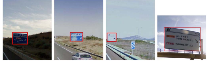
Fig. 6. Correct panel detection under illumination changes.
