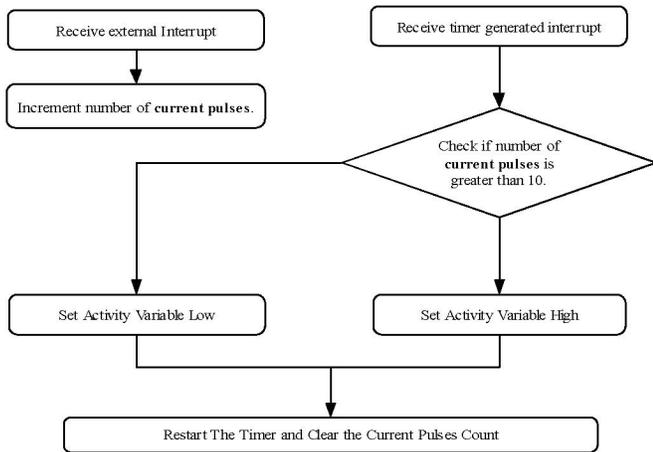
Figure 4. Algorithm for load detection
