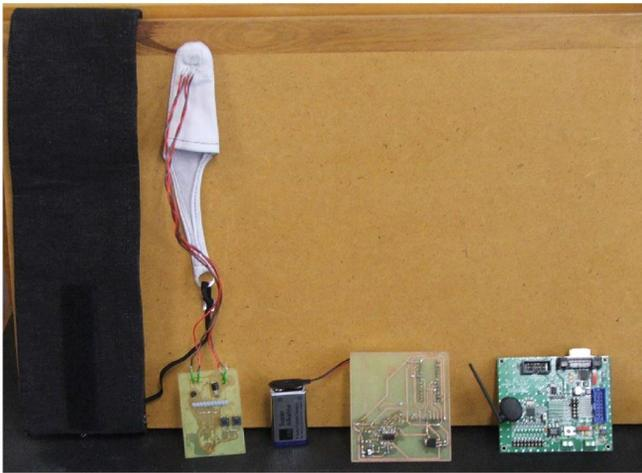
Figure 10. Device prototype and finger glove
