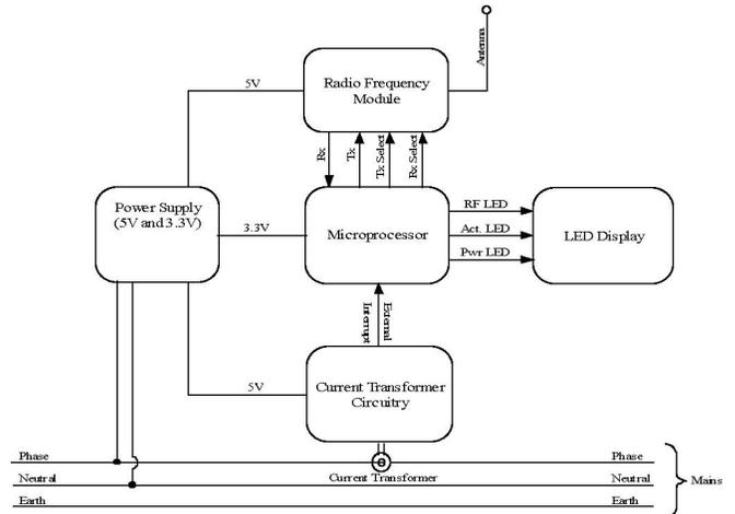
Figure 3. Core components of the Sensor Unit (SU)
