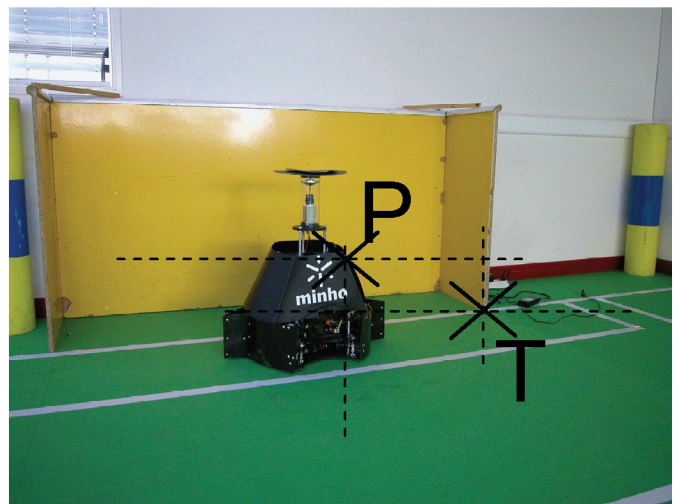
Fig. 2. Example of image with localization of optical centre P and target T
